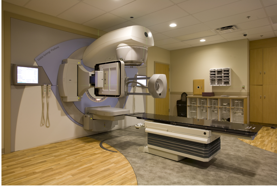
Figure 3.2.1: An Elekta radiation treatment machine (Capital Radiation Therapy (2013)) with an x-ray imager mounted.
